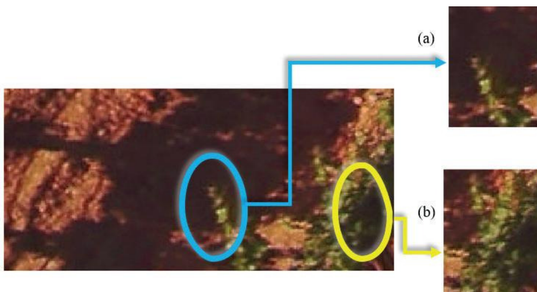
FIGURE 12. Shadow recognition issues: (a) vegetation over the shadows, and (b) shadows in the vegetation.
