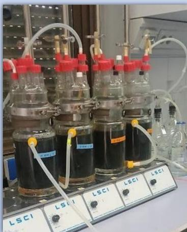
The experiments were conducted in 1 liter reactors (Figure 1) with a mixture substrate/inoculum 1:1, (in VS proportions).
